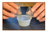
6. Mix by "folding" the resin and hardener together for two minutes; scrape the sides of the cup as you mix.
