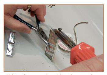
Holding the piece steady with bent chain nose pliers. Since flux can damage tools, and you may drip solder onto them, dedicate an inexpensive or already damaged pair for use in soldering.
