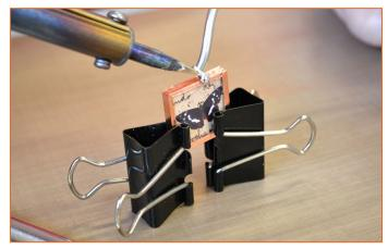
Adding solder to the tape. Use binder clips to hold piece in place while you hold the spool of solder in one hand, and the iron in the other.
