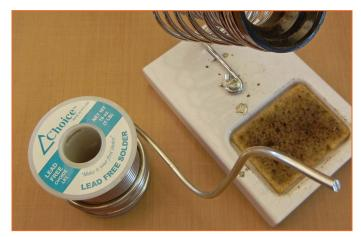
Shaping the solder coil into a snake makes it easier to feed onto your soldering iron
