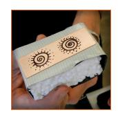
6. Cover all areas that should not be etched with ink or durable tape. This includes the back, sides and inside any holes.
